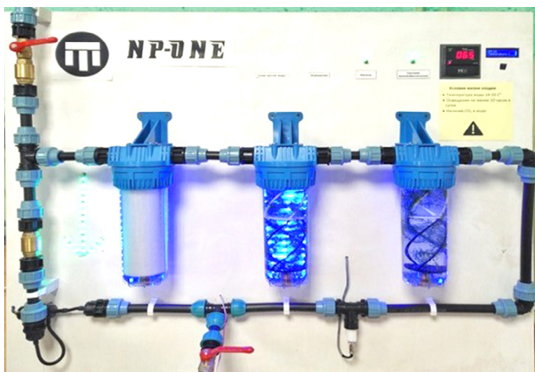
Figure 1. The water purification machine assembled by schoolchildren
